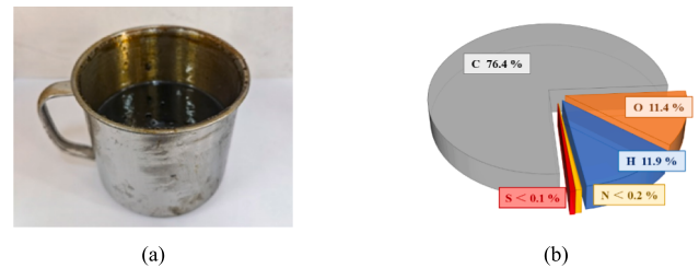
Fig. 5. Image and elemental analysis of bio-oil (a) Appearance; (b) Elemental composition.
