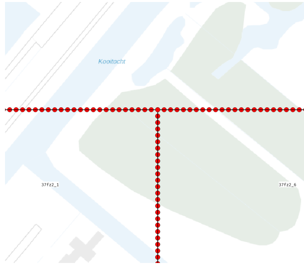
Figure 2.3: Steiner points being added along sub-tile borders to enforce common triangulation points. Figure from Dukai [2020].
