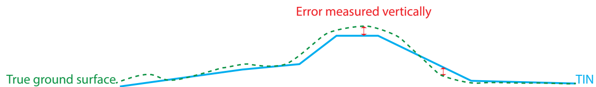
Figure 4.2: Figure showing that error is measured vertically and how a TIN subsequently approximates the real surface. Adapted from Ledoux et al. [2021b].
