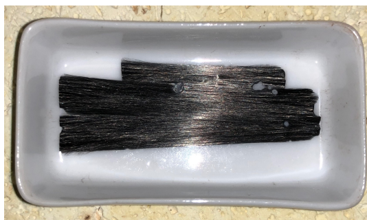
Figure 4.18: Pure carbon fibers after degradation of the PPS matrix
