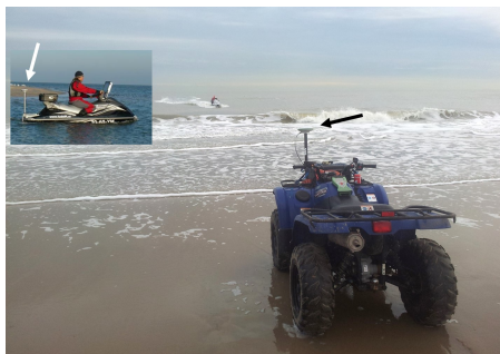
Figure 16.3: Both the on- and offshore part are regularly surveyed, to monitor the development of the Zandmotor (The Sand Engine), at the Dutch North-Sea coast, near Ter Heijde. This 'building with nature' project started in 2011, and at right an aerial photo of the Zandmotor is shown, looking in Southern direction. High-precision RTK-GPS is used for positioning the quad on shore, and the jet-ski in the water (note the GPS-antenna at the back of the jet-ski, in the inset). The measurements by the quad result in a Digital Terrain Model (DTM), and echo sounder depth measurements by the jet-ski result in a seafloor-map. Photo at left by Matthieu de Schipper [42]. Photo at right by Pmbloom - own work, May 2016, taken from Wikimedia Commons [9] under CC BY-SA 4.0 license.
