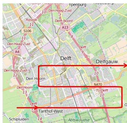
Figure 19.8: Example of flight trajectory to map the TU Delft area through stereo-photogrammetry, using the principle of Figure 19.7. A 7 km by 7 km area is shown. The area is flown strip-wise, and the parallel tracks are about 1.2 km apart (turns of the aircraft are not shown realistically). With a flying-height of over 4 km, the footprint of one photo on ground is typically about 1.3 km x 2 km. The background map is taken from OpenStreetMap (OSM) , ©OpenStreetMap contributors [51], cf. Appendix J.
