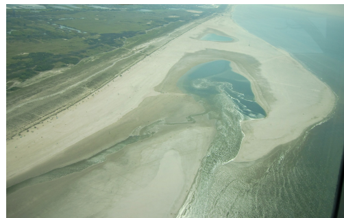
Figure 16.3: Both the on- and offshore part are regularly surveyed, to monitor the development of the Zandmotor (The Sand Engine), at the Dutch North-Sea coast, near Ter Heijde. This 'building with nature' project started in 2011, and at right an aerial photo of the Zandmotor is shown, looking in Southern direction. High-precision RTK-GPS is used for positioning the quad on shore, and the jet-ski in the water (note the GPS-antenna at the back of the jet-ski, in the inset). The measurements by the quad result in a Digital Terrain Model (DTM), and echo sounder depth measurements by the jet-ski result in a seafloor-map. Photo at left by Matthieu de Schipper [42]. Photo at right by Pmbloom - own work, May 2016, taken from Wikimedia Commons [9] under CC BY-SA 4.0 license.
