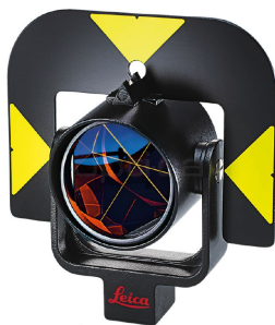
Figure 4.11: Corner cube reflector for EDM measurements with a total station (Leica survey prism GPR121). The reflector can be mounted on a range pole and taken to survey points of interest, or by means of a carrier installed on a tribrach on a tripod.
