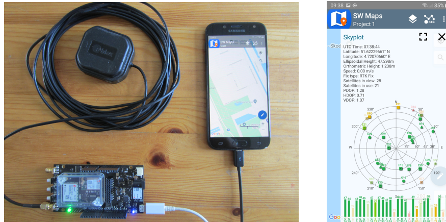
Figure 15.7: At left: dual-frequency, multi-constellation GNSS receiver with receiver board at bottom, small patch-antenna (black) on top, and smartphone with Android positioning app at right; a total equipment cost of below 500 Euro (u-blox ZED-F9P), yet capable of providing cm-accurate RTK-GNSS positioning. At right: screenshot of SW Maps app by Softwel (P) Ltd.
