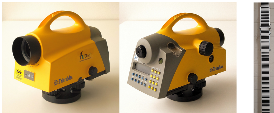
Figure 3.10: A modern electronic automatic level with digital read-out and data-logging functionality, Trimble DiNi 12. At right (a part of) the so-called bar-code rod or staff is shown, to be used with this digital leveling instrument.
