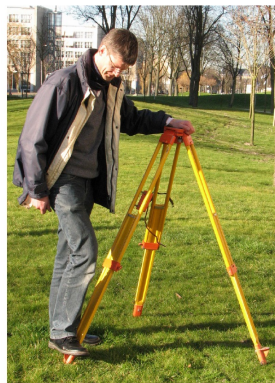
Figure 3.17: Fixing the tripod legs on soft ground.
