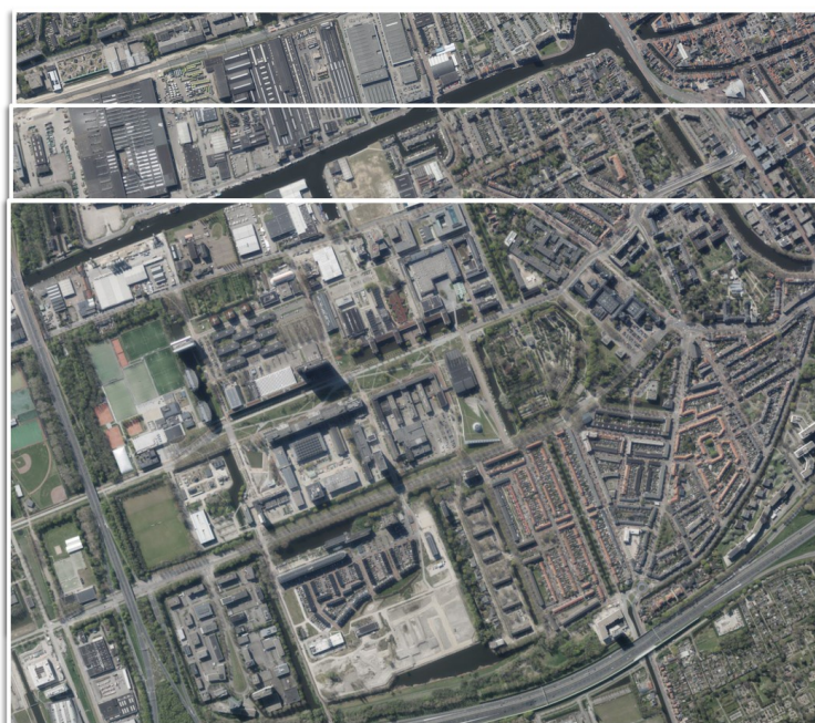
Figure 19.9: Example of three overlapping photos in one strip, for the purpose of mapping the TU Delft campus area through stereo-photogrammetry. The photos have been taken with a Vexcel Ultracam Eagle Mark 3 camera (450 Megapixels), with a focal-distance of f=210 mm, at a flying height of slightly over 4 km. Photos obtained through Beeldmateriaal Nederland [49] under a CC BY 4.0 license.
