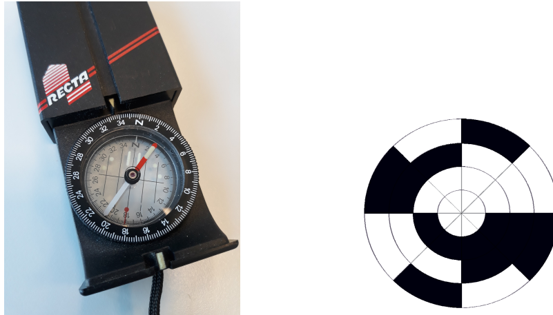
Figure 18.1: At left: magnetic compass for hiking or sailing with a 360-degrees-scale divided in 2-degrees portions. At right: 360-degrees disc divided in three rings, with each ring in total half of it being black and half white; in this example directions are encoded using (only) 3 bits; when a full turn of 360 degrees is divided by 2^3 different codes, this yields a 45 degrees resolution for the measurement of direction.
