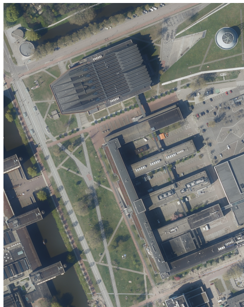
Figure 19.1: Example of an aerial photograph of a part of the TU Delft campus, taken April 26th 2021, with a Vexcel Ultracam Eagle Mark 3 camera (450 Megapixels), with a focal-distance of f=210 mm, and a flying height of slightly over 4 km. Shown is an orthophoto with a ground pixel resolution of 8 cm. Aerial photographs are jointly acquired in the Netherlands, country-wide, by a cooperation of Dutch governmental bodies, led by het Waterschapshuis and het Kadaster, for instance for mapping purposes through stereo-photogrammetry (for example the Basisregistratie Grootschalige Topografie (BGT)). Photo obtained through Beeldmateriaal Nederland [49] under a CC BY 4.0 license. From 2021 on, these aerial photos are available as open data.
