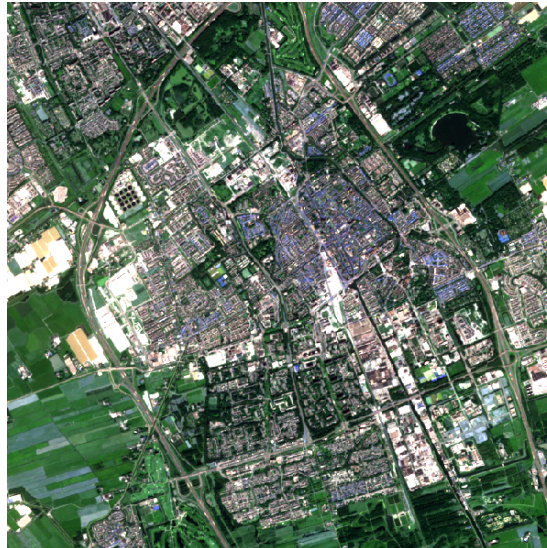
Figure 25.4: 'True color' image, created by combining the three images of Figure 25.3. Data from ESA Sentinel-2 satellite (Copernicus Sentinel data 2019) obtained through Sentinel-Hub [1], CC BY-NC 4.0, covering the area of Delft, 7 km x 7 km, with the old city center in the middle, and North up.
