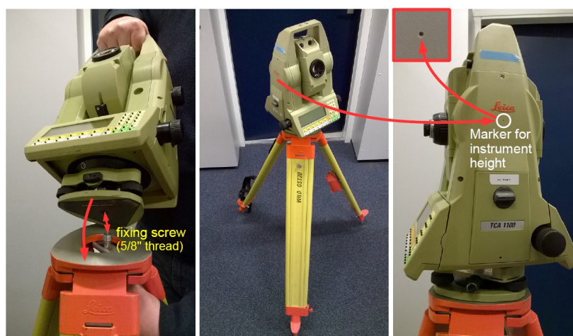
Figure 4.20: Mounting a total station on a tripod. Note, in the photograph at right, the marker on the instrument to measure the height of the instrument above the benchmark in the ground. The marker on the instrument coincides with the horizontal axis. The instrument height should be measured, with a tape, once the instrument set-up has been completed.
