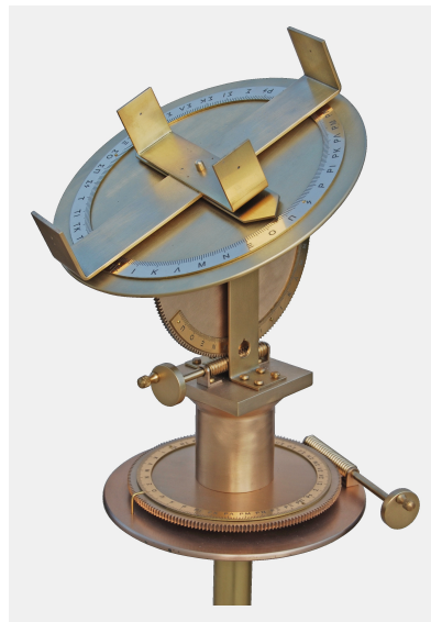
Figure 2.3: The dioptra described by Heron of Alexandria. Image courtesy of Kotsanas Museum of Ancient Greek Technology, Katakolo, Ilia, Greece, [13].
