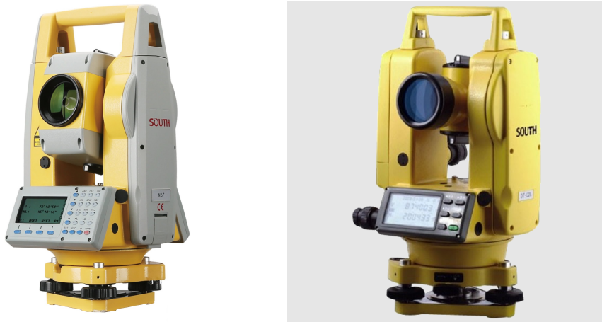
Figure 2.9: At left an example of a modern total station (South 6N+), and at right a modern theodolite (South DT-02L). The theodolite at right looks more lean, and has a display showing just vertical and horizontal angle. With the total station at left much more electronics is involved, in particular for the built-in Electronic Distance Meter (EDM). Photos courtesy of South Surveying and Mapping Technology Co., Ltd. [19].
