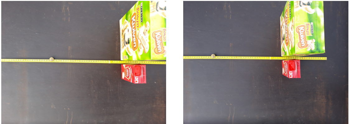
Figure 19.10: Stereo-photogrammetry at home: the same scene is pictured twice, with a smartphone camera (Samsung J5 2018 - SM-J530F). The camera was held (approximately) level, at a 'flying height' of 60 cm.
