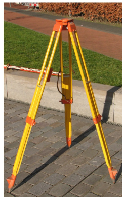
Figure 3.18: Fixing the tripod legs on hard surface.
