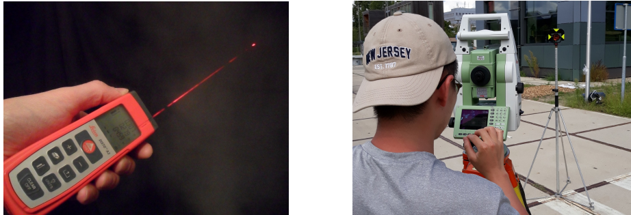
Figure 18.6: Both a laser distometer (at left) and a total station (at right) use two-way ranging, generally by means of a laser. The laser distometer (shown here) uses red laser light with a 635 nm wavelength for ranging with millimeter precision, on distances up to 30 meters. The distance is measured optically, using a pulsed laser as an emitter, and a photo detector as a receiver (integrated in the same device; the two-way traveltime of the laser pulse is measured). Pulses, with a duration ranging from a few to several tens of nanoseconds, are repeatedly transmitted, with a repetition rate in the order of kHz. The laser light of the distometer reflects directly on the object of interest. With a total station often a reflector is used, as shown at right.
