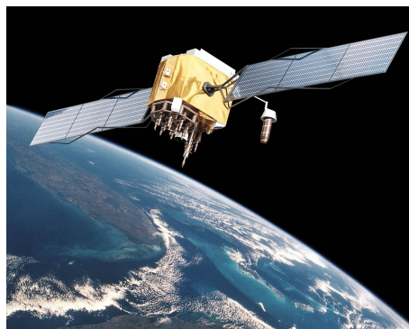
Figure 12.1: GPS block IIF satellite, built by Boeing. These GPS satellites, 12 in total, have been launched between 2010 and 2016. They have a design lifetime of 12 years. The full GPS constellation nominally consists of 24 satellites. Image courtesy of Boeing [33].
