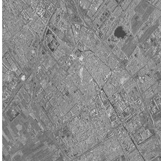
Figure 20.4: Example of radar amplitude image. Amplitude per pixel is shown in gray-scale from black to white. The image shows the area of Delft, about 7 km x 7 km, with the old city center in the middle, and (approximately) North up, acquired, on Nov 1, 2015, by the DLR TerraSAR-X satellite [53] at 500 km altitude. The data are available with a pixel size on ground of about 3 m x 3 m. Water bodies, like the Schie-canal, typically show up in black.
