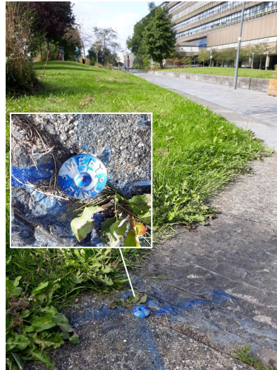
Figure 14.7: Survey-marker at TU Delft campus with accurate ground-truth coordinates: X = 3923768.0147 m, Y = 300255.7048 m, Z = 5002640.2228 m (ITRF2014 at epoch 2021.50).
