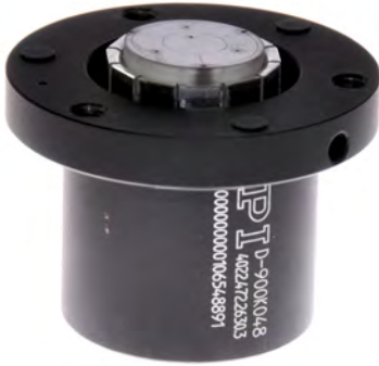
(a) The ASML/PI TSA mounted in its housing. This housing acts not only as a means to mount the sensor and the actuator, but it also reduces the displacement sensitivity to environmental temperature changes, by placing the electrode in the thermal centre. (The housing and the fingers expand equally, reducing the electrode motion due to environmental temperature changes.)
