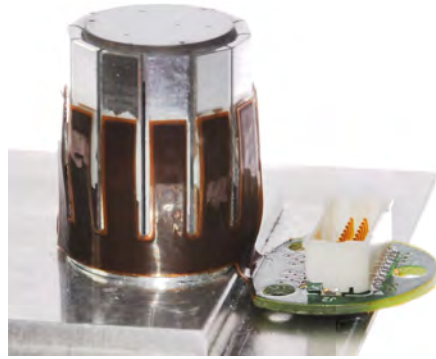
(b) The ASML/PI TSA with the partial flexible PCB and heaters exposed. The actuator is mounted to an aluminium block that acts as a heat sink. The experiments discussed in this thesis use this mounting method to achieve better thermal conduction to the environment.
