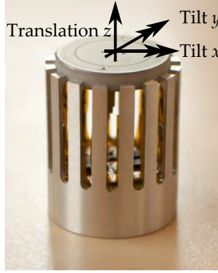
Figure B.3.: Axis definitions of the TSA in three degrees of freedom: tilt angles x and y and translation axis z .
