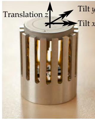
Figure 4.14.: Axis definitions of the TSA in three degrees of freedom: tilt angles x and y and translation axis z .
