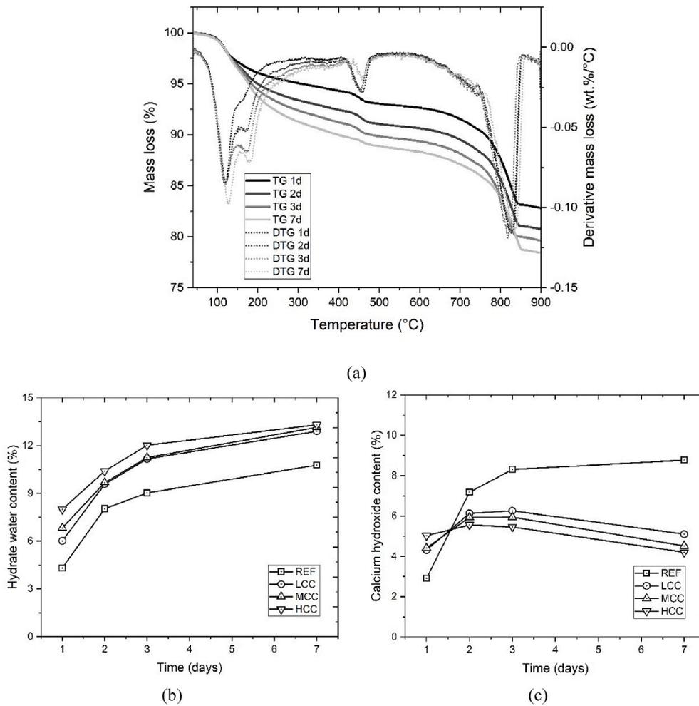
**Fig. 19.** TGA at 1, 2, 3, and 7 days: (a) a typical example of TG and DTG curves (mixture HCC); (b) The normalized amount of hydrate water (H) relative to the dry sample weight at 600 °C; (c) The normalized amount of calcium hydroxide (CH) relative to the dry sample weight at 600 °C.
