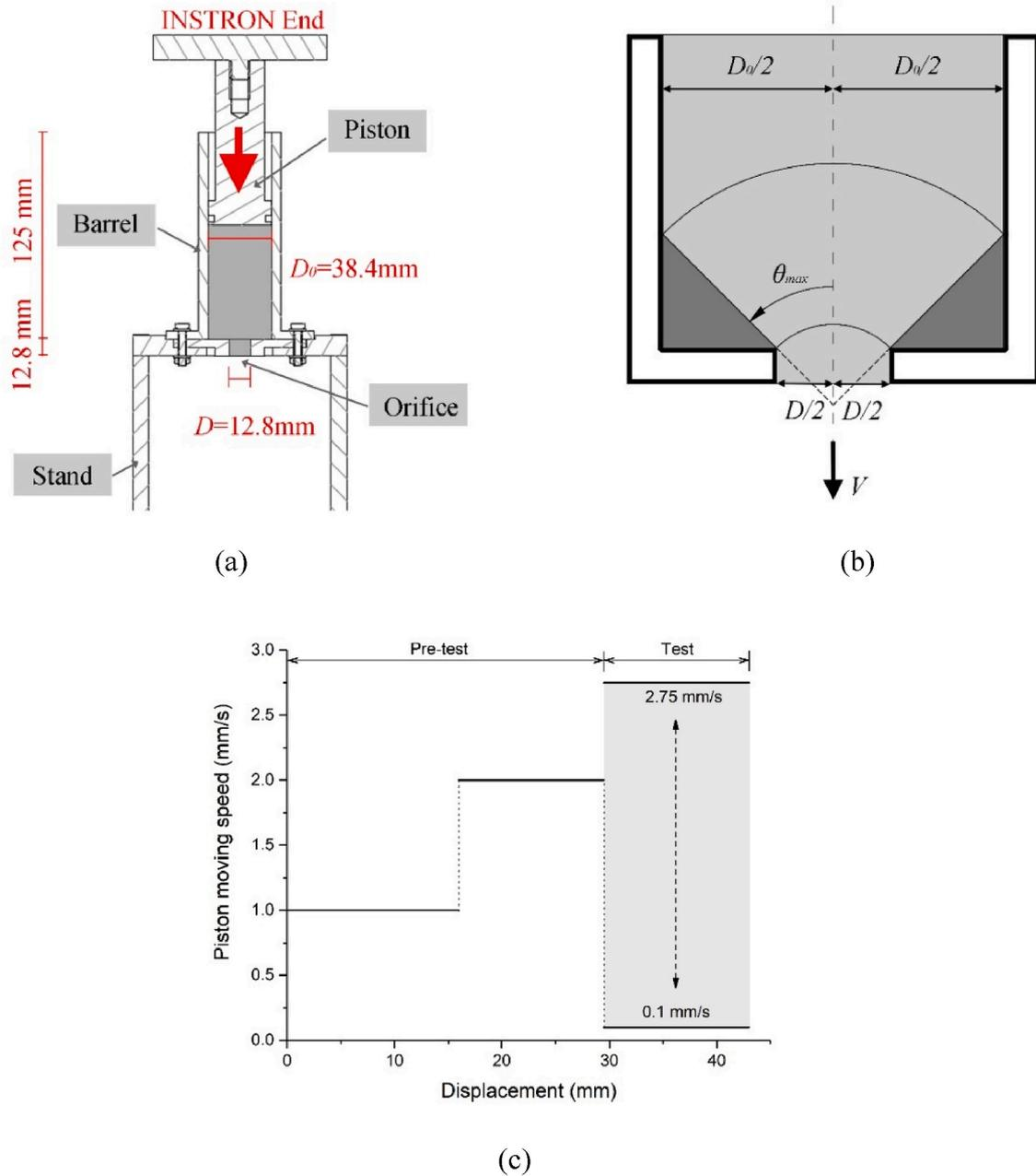
Fig. 5. (a) Schematic drawing of the ram extruder; (b) Diagram of the orifice entrance flow region in a spherical coordinate system, according to Ref. [26,27]; (c) A typical trial of the ram extrusion test - predefined piston moving speed vs. displacement.
