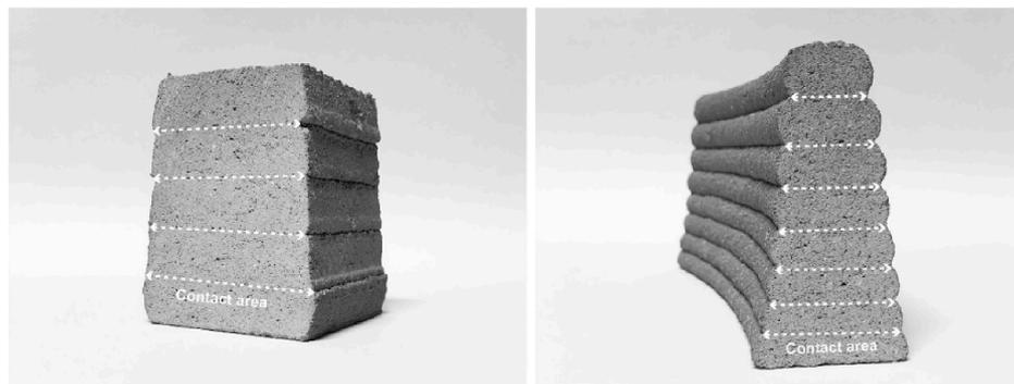
Fig. 15. Cross-sections of printed samples by using nozzle 1 (left) and nozzle 2 (right). The dashed line represents the contact area between two adjacent layers.
