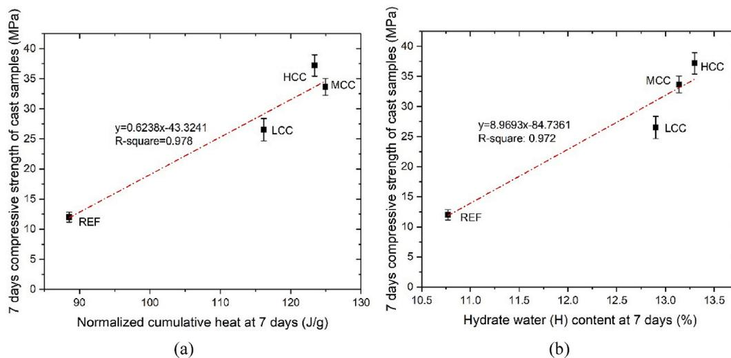
**Fig. 22.** The linear relationship between 7 days compressive strength and (a) Normalized cumulative heat at 7 days (excluding any heat within the first 12 h after mixing) obtained from isothermal calorimetry test; (b) Hydrate water (H) content at 7 days obtained from TGA.
