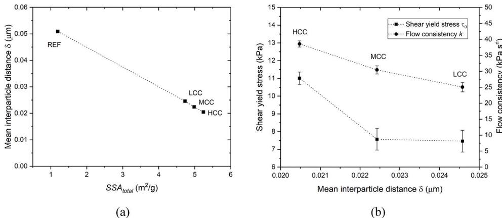
Fig. 20. Relationship between (a) Mean interparticle distance and total SSA of solid; (b) Mean interparticle distance and shear yield stress as well as flow consistency obtained in Section 3.1.
