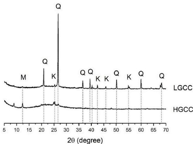
Fig. 1. XRD patterns of LGCC and HGCC. Q-quartz (SiO<sub>2</sub>), M-mullite (3Al<sub>2</sub>O<sub>3</sub>·2SiO<sub>2</sub>), and K-kaolinite (Al<sub>2</sub>O<sub>3</sub>·2SiO<sub>2</sub>·2H<sub>2</sub>O).
