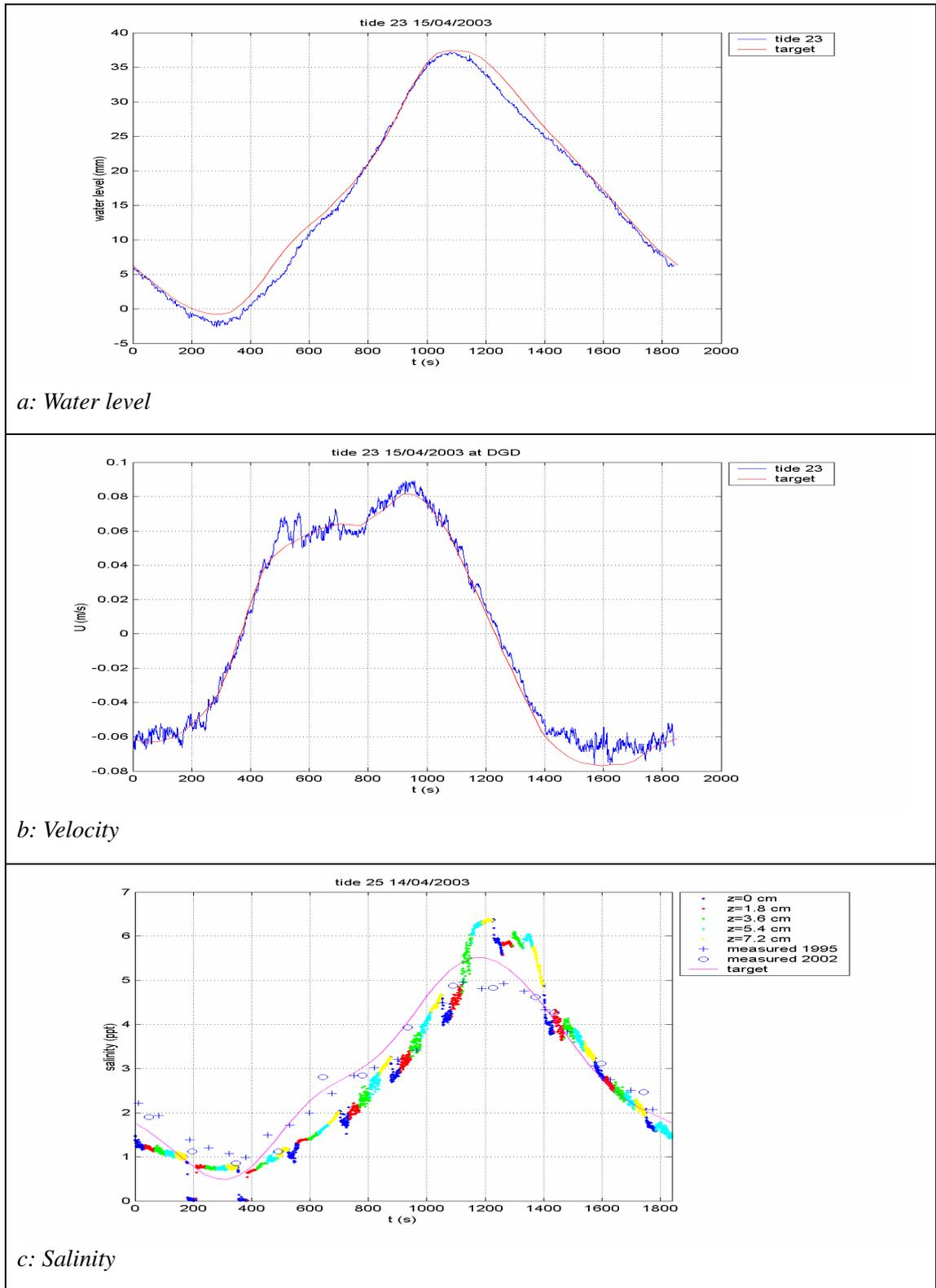
Figure 5.5: Calibration results for the physical scale model (van Kessel and Cornelisse, 2003).
