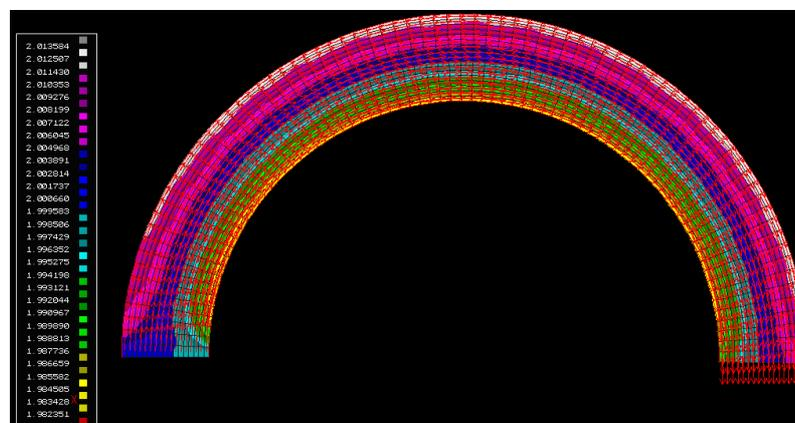
Figure 5.15a: Velocity distribution in river bend with ‘ideal’ circular grid
