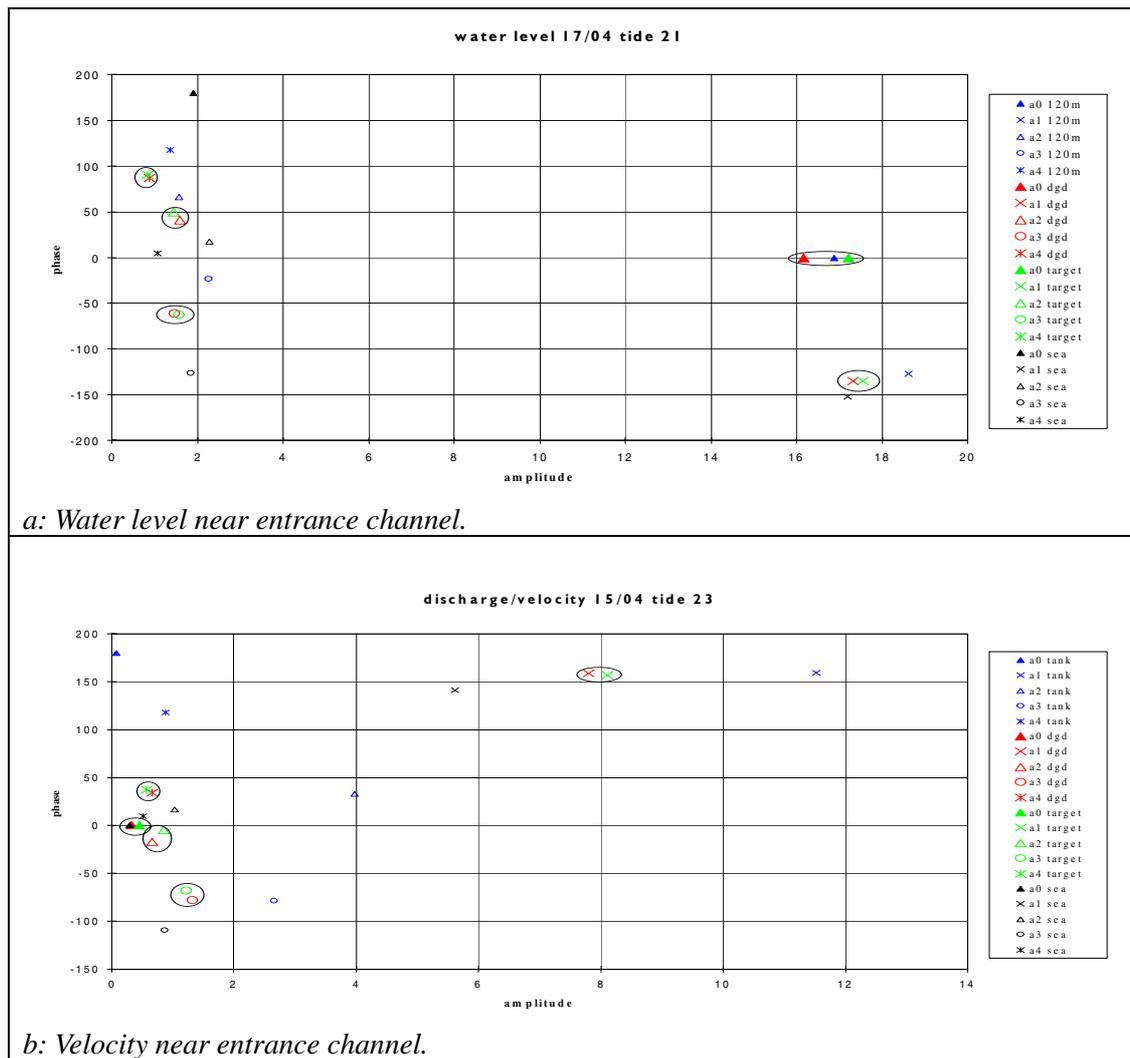
Figure 5.6: Amplitude-phase diagrams.
