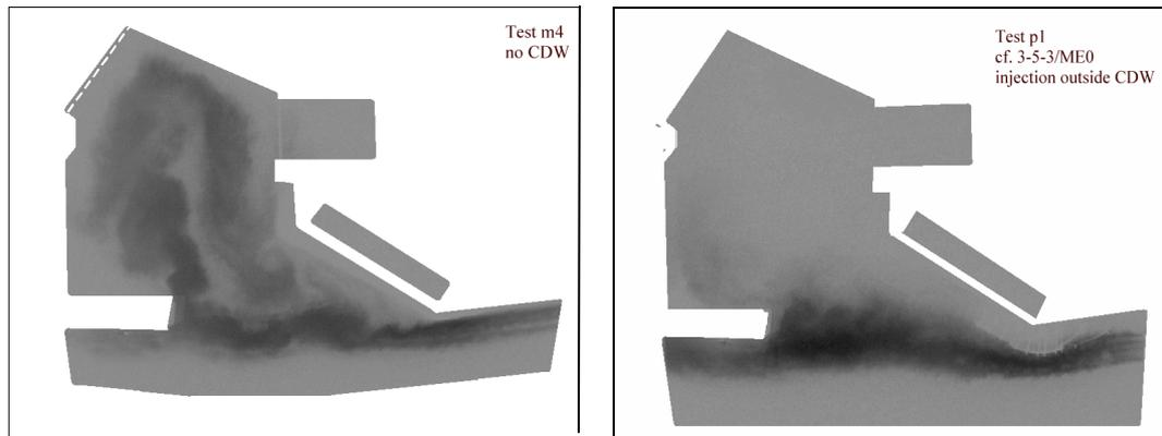
Figure 2.6: Dispersion of dye in the Parkhafen 700 s (model time) after start of dye injection upstream of the harbour entrance during flood. Left panel: without CDW; right panel: with CDW and dye injection at the outside of the CDW.
