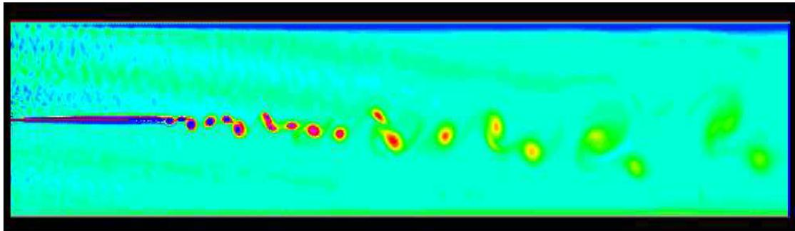
Figure 4.2: DELFT3D simulations: mixing layer due to velocity differences between upper and lower layer (figure is slightly distorted).
