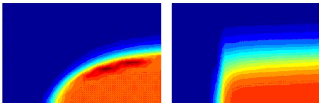
Figure 5.13: Characteristic salinity distribution (side view) of the front of a gravity current; non-hydrostatic model (left) and hydrostatic model (right) (Bijvelds, 2003).
