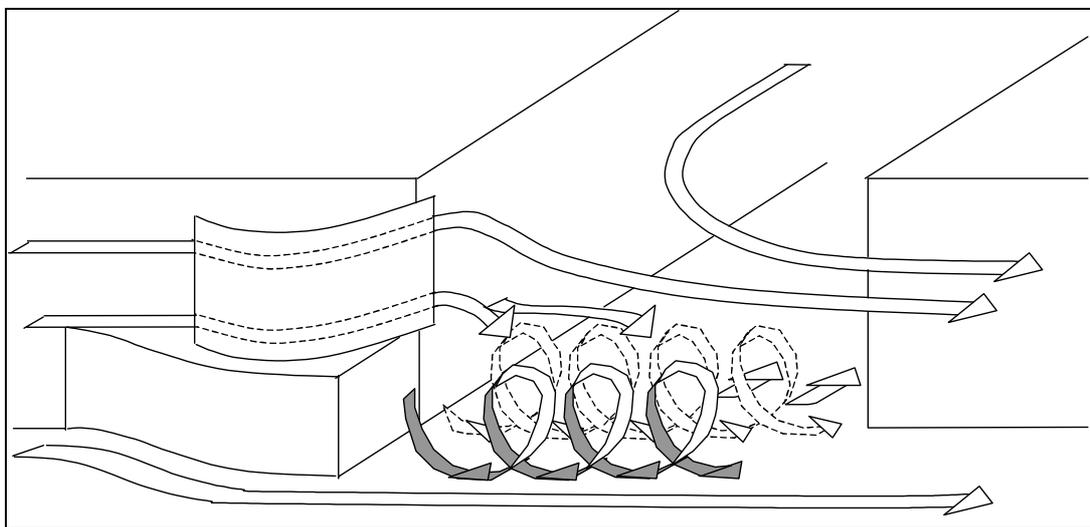
Figure 2.2. Schematic helical flow pattern in entrance during flood, with CDW present (non-homogeneous flow conditions).
