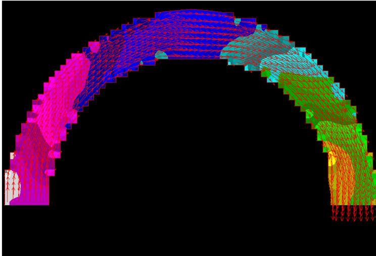
*Figure 5.15b: Velocity distribution in river bend with rectangular grid without smooth boundary approximation*
