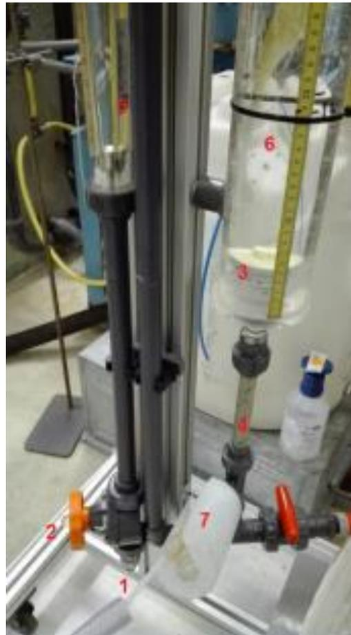
Figure 16 Displays the used PFR. Hard water flows in (1) as the valve (2) is turned to a certain discharge, which is read at an venturi meter (5). NaOH is mixed with incoming hard water (7) and goes through a static mixer (4). Finally it is brought via a mixing h (3) into the 1 m column (6) (Seepma, 2018)
