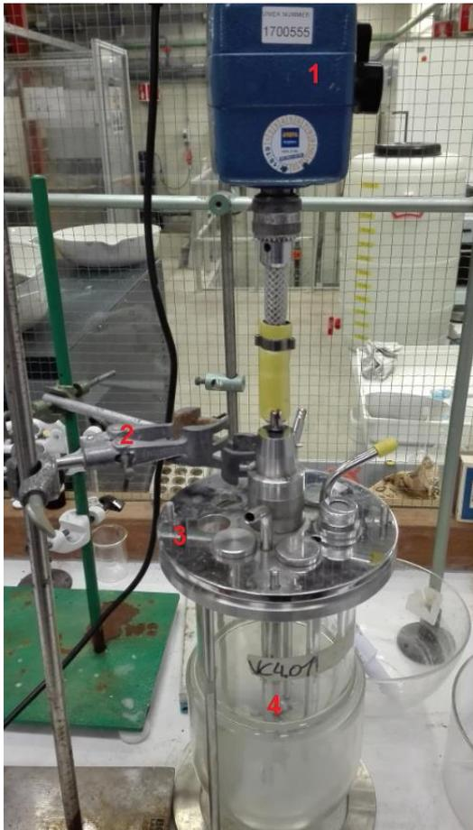
Figure 15 Experimental setup of the CSTR. The agitator's generator (1) is connected onto the top of the CSTR, which is attached to the RVS agitator (4). The pH and EC probes are then held by arms (2) into the solution. Finally NaOH is added through one of the holes present (3) in the lid and the holes are sealed off accordingly (Seepma, 2018)
