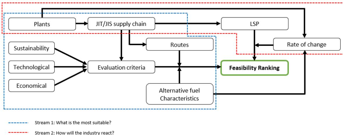
Figure 1: Conceptual model for the feasibility ranking of alternative fuels in a JIT/JIS supply chain
