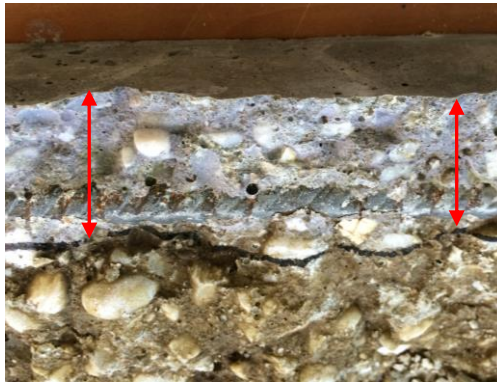
Figure 5-24: Chloride penetration in concrete cube after two years of exposure
