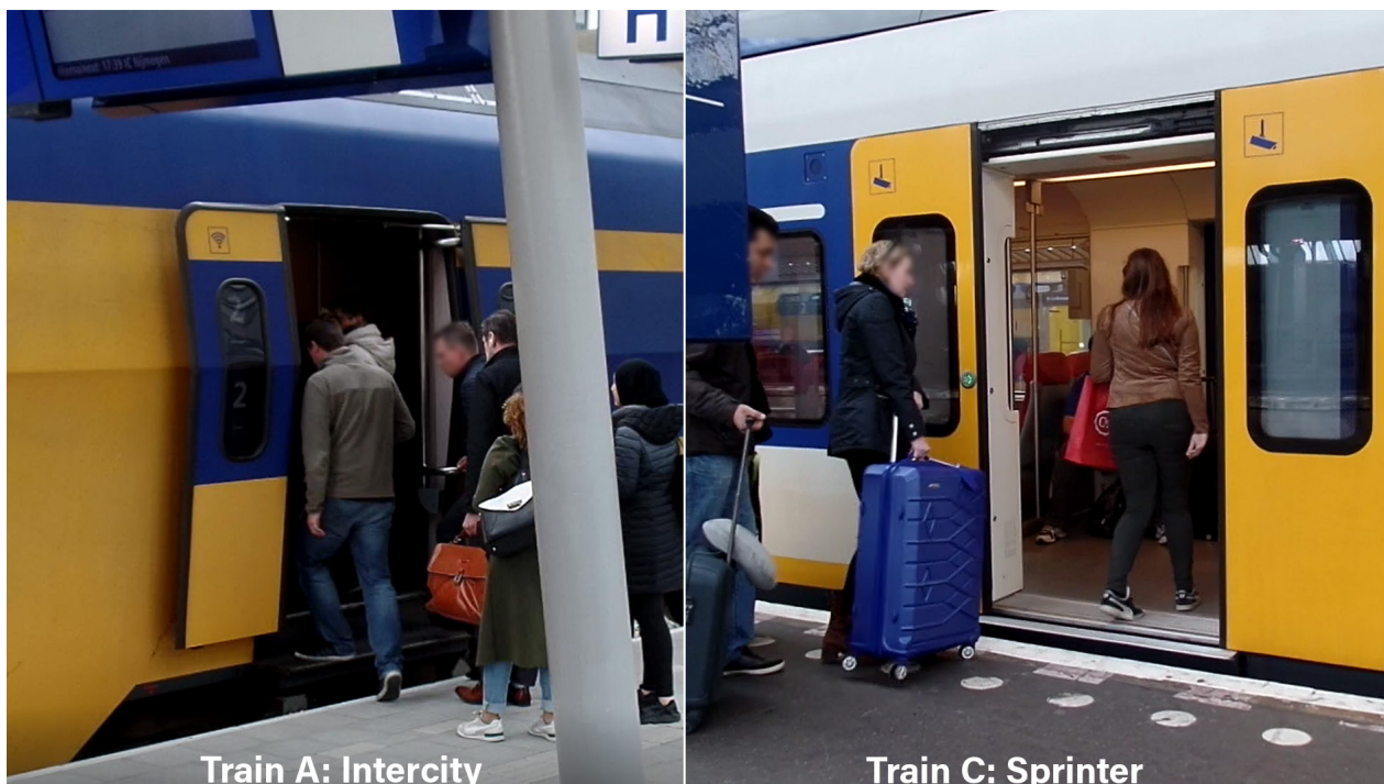
Figure 14. Two types of trains observed (A: narrow doors and stairs; B: wide doors and no stairs).
