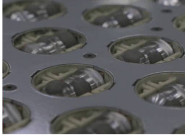
▲ Figure 46. Omnidirectional conveyor belt units.
