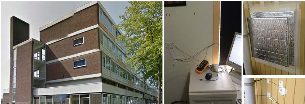
Figure 10.3: Case study 3- The whole building (left), the inside surface of the wall (middle), and the outside surface and sensors covered by the box (right). Location: Delft, the Netherlands.
