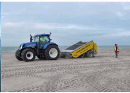
Figure 37. Beach cleaning machine, used as mechanical aid in combination with hand picking.
