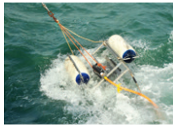
Figure 32. Shallow seismic device 'Boomer' floating on surface towed next to the fishing boat while searching for finds.
