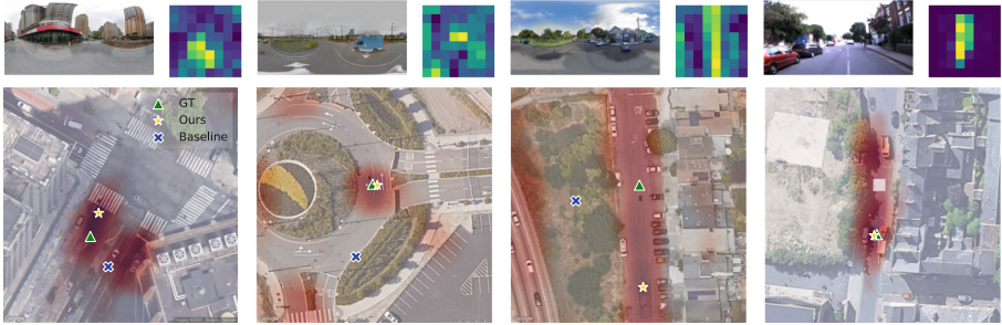
Fig. 4. Top: input ground images and matching score maps at the model bottleneck, bottom: input satellite image overlaid with outputs from CVR and our method. From left to right: 1: VIGOR, same-area, 2,3: VIGOR: cross-area, 4: Oxford RobotCar.
