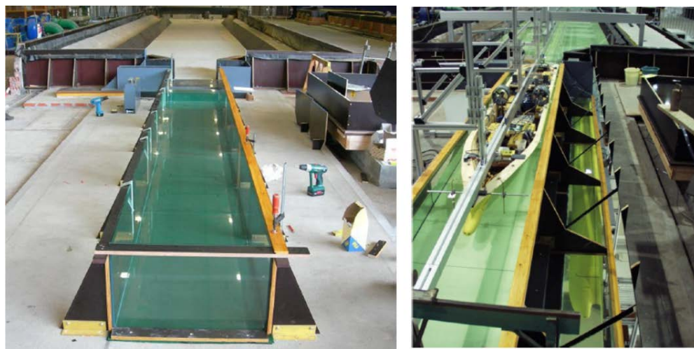
Figure 4.14: Overview of the physical scale model of the new IJmuiden sea lock (source: Deltares).
