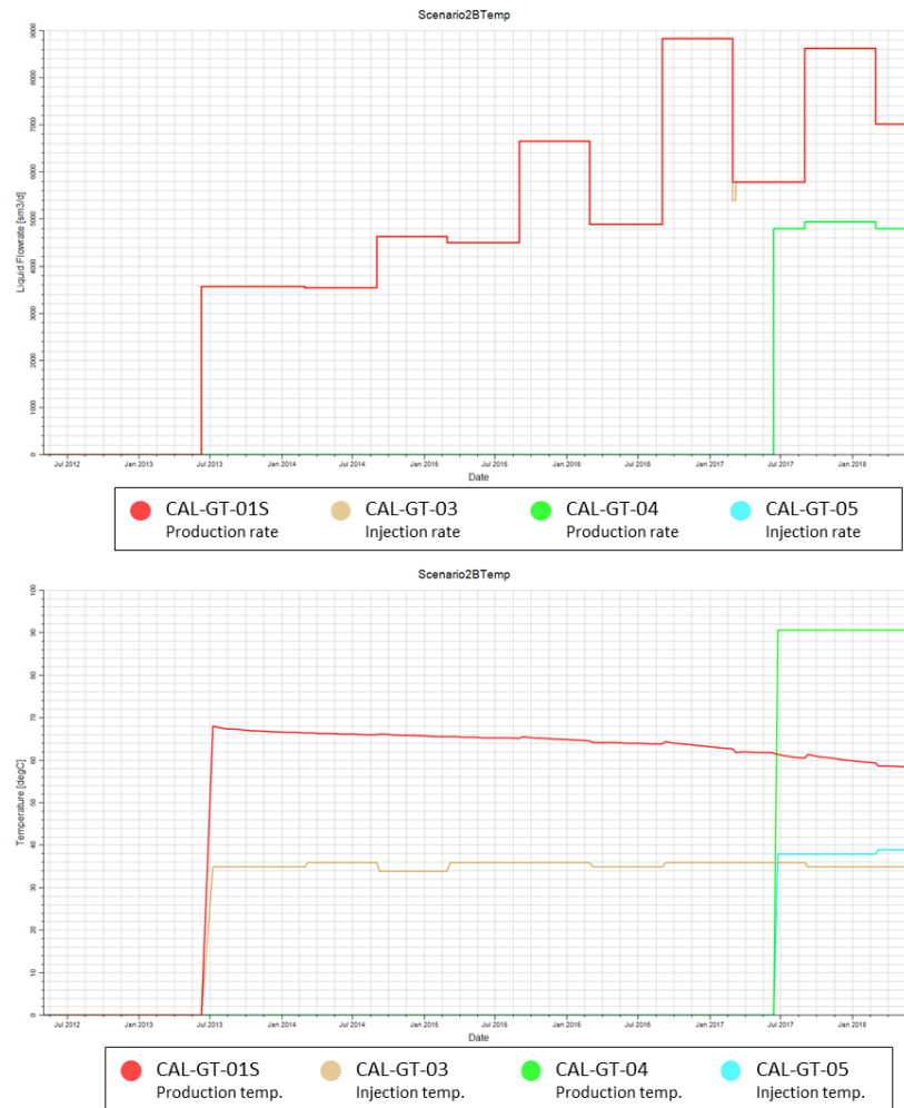
Appendix E. 17. Case: Scenario2BTemp. BHP, flow rate and temperature plot of Scenario2B* with a small radius (370m) and a high permeability value ( K_j=7 D)
