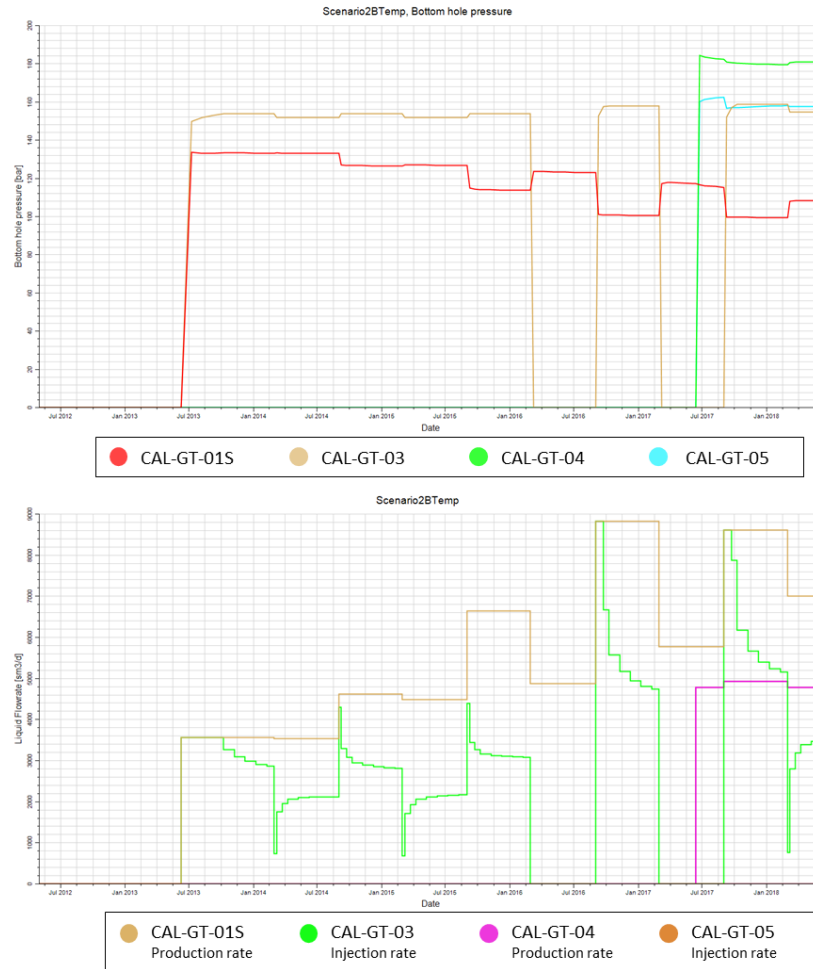
Appendix E. 16. Case: Scenario2BTemp. BHP and flow rate plot of Scenario2B* with a small radius (250m) and a high permeability value ( K_j=12 D)
