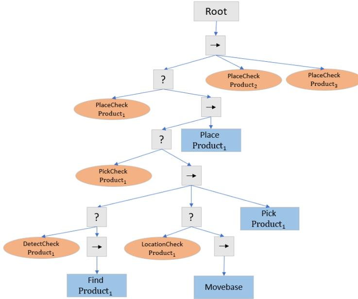
**Figure 6:** Example of BT generated to prepare a list of products, focusing on one product BT expansion, full BT generated and executed can be seen in the Appendix in Figure 3
