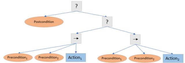
**Figure 1:** Template for an atomicBT with multiple actions to satisfy the same post-condition
