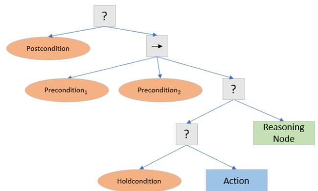
**Figure 3:** Template for atomicBT of skill with a fallback branch or hold-condition
