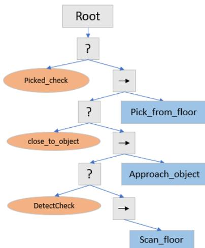
**Figure 8:** Final iteration for the generated recovery behaviour for the goal condition Picked\_check, the generated BT for the recovery behaviour can be seen in the appendix Figure 5b.
