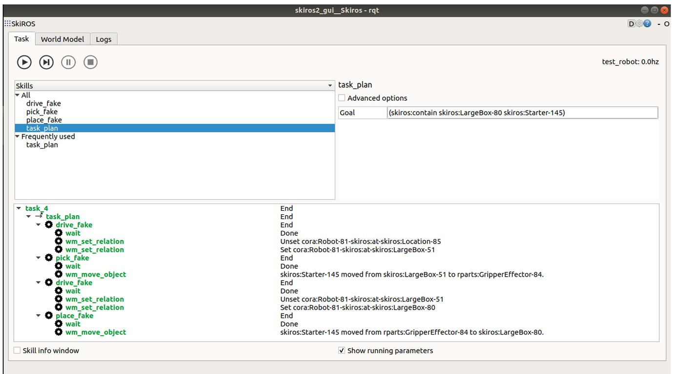
Figure 1: SkiROS GUI executing the plan for the kitting task
