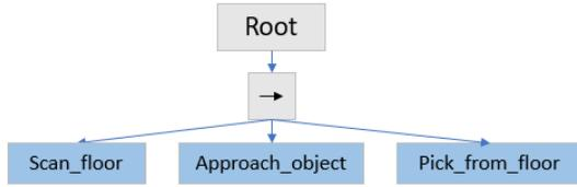
**Figure 7:** Fallback branch to recover from dropping the product, the branch used can be seen in appendix Figure 5a.
