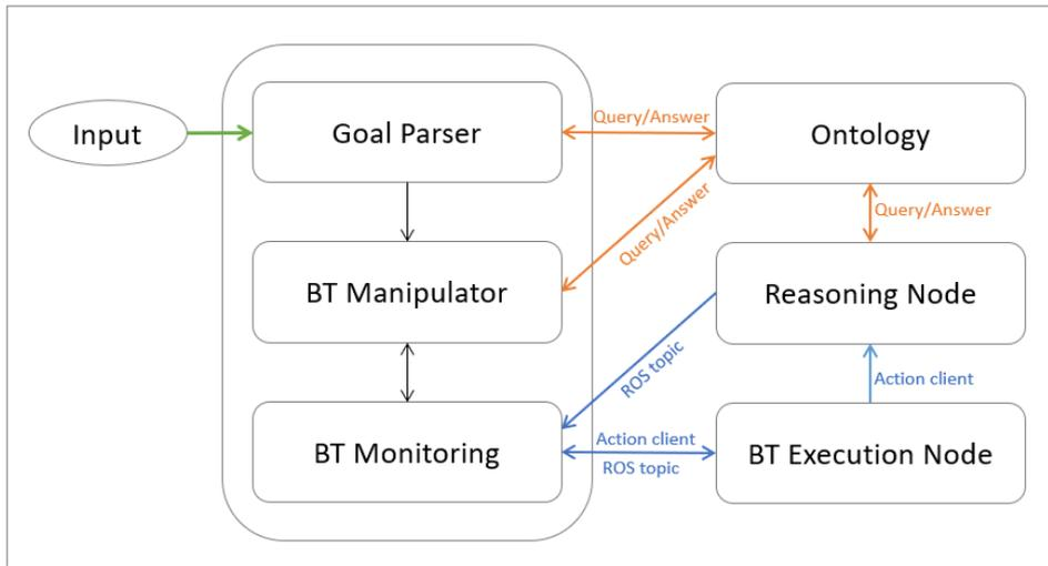
**Figure 2:** The connections between the main components of FROGBT's architecture
