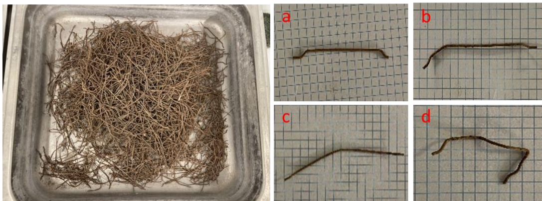
Fig. 1 The recovered steel fibre (left); types: a. Complete; b. Others; c. Angle < 90 degrees; d. Angle > 90 degrees (right)
