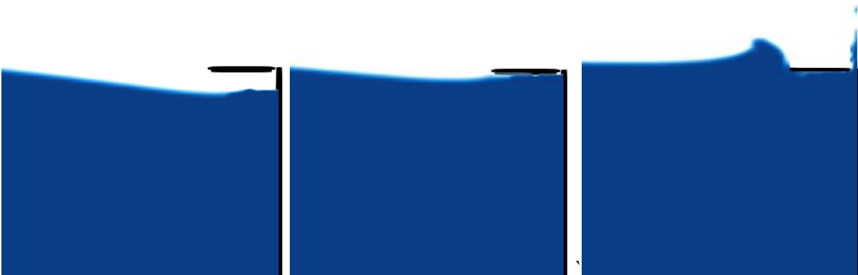
Fig. 8. Snapshots of water body just before, during, and after impact of a regular wave on an overhang ( O/W = 0.1 , W/G = 1/6 , L/W = 24 , h/L = 0.25 , H_i/L = 0.025 ). Only a part of the domain around the overhang is shown.
