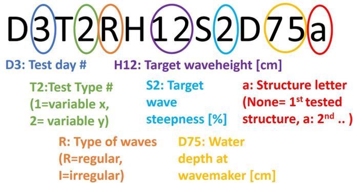
FIGURE 3.6: Explanation of abbreviations used in the test codes
