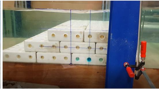
(H) Structure 2 - holes blocked with pipes
