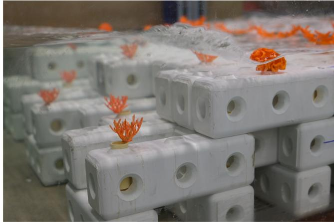
FIGURE 3.5: Close-ups of one of the Reefy design configurations tested during the experiments for this thesis. The 3D-corals are added to investigate the effect of increased surface roughness once reef-building species colonize or are pre-seeded on the structure.
