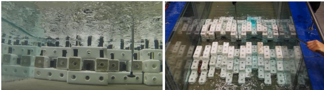
(A) Picture taken in the flume of EVM behind structure 8-I
