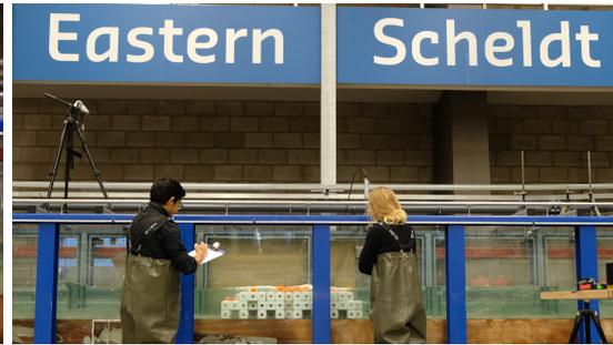
(B) Set-up around the flume (top camera+observation form)
