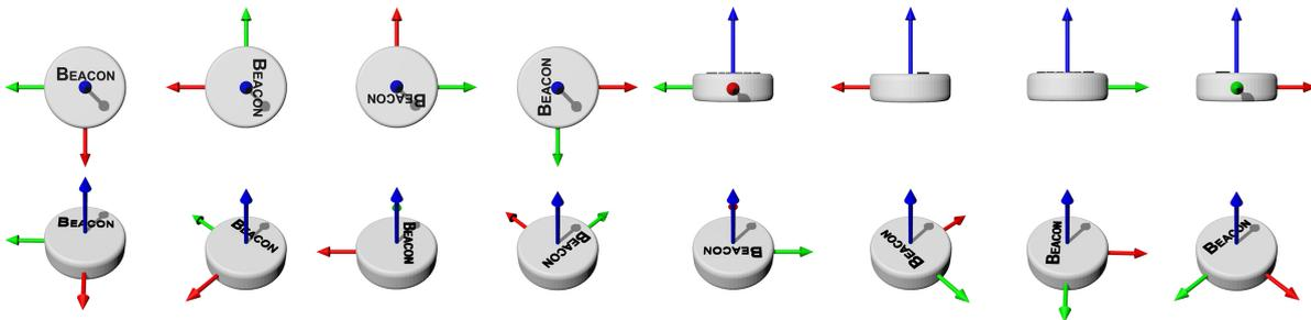
Figure 2.11: Beacon orientations that were tested
