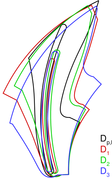
Figure 6.19: Geometry comparison between preliminary ( D_{p,l} ) and optimized ( D_1 , D_2 , D_3 ) vane diffusers for the three-dimensional Reynolds averaged Navier-Stokes multi-objective optimization with larger impeller.
