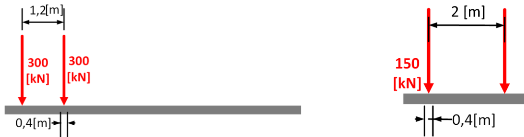
Figure 2.15: Axle and wheel distribution Eurocode. On the left a cross-section in length direction, which shows the division of axle loads on a single lane. On the right a cross-section in width direction, which shows the division of the axle loads over the wheels. The distances between the axles and wheels are indicated and the size of the contact area is indicated in the bottom of the picture.
