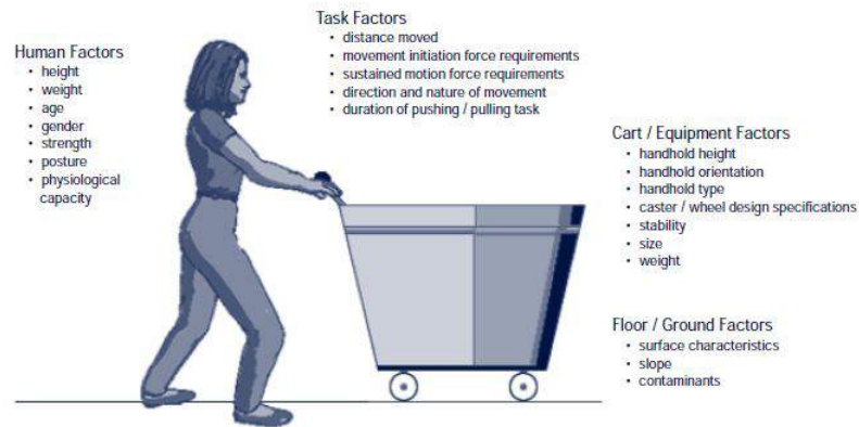
Figure 2-3: Factors influencing a human while pushing an object [13].
