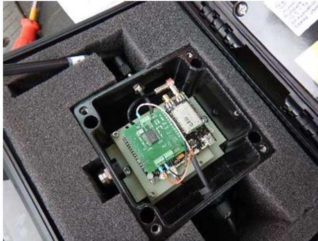
Figure 11.22 Hardware components in LoRaWAN sensor node prototype, embedded in an ATEX compatible chassis. Source: Eawag.
