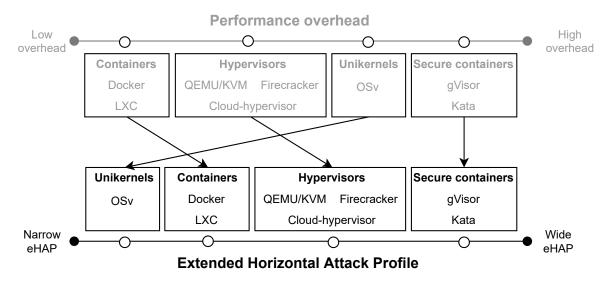
Figure 6.6: Mapping of performance overhead to extended HAP per isolation platform category. Performance overhead is displayed in gray as it is also shown in Figure 5.23
