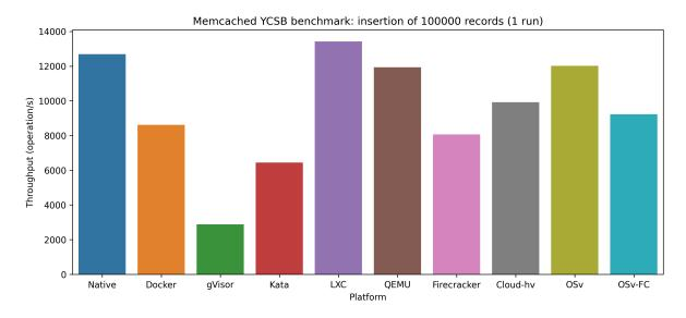
Figure A.6: Memcached YCSB benchmark, insertion stage (100000 records)
