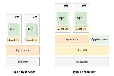
Figure 2.1: Architecture of type-1 vs. type-2 hypervisors
