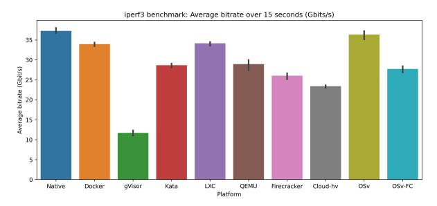
Figure 5.15: iperf3 network throughput benchmark, maximum throughput achieved.
