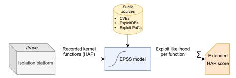
Figure 6.2: Extended HAP pipeline
