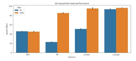
Figure 5.12: dd read throughput
