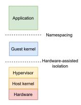
Figure 6.11: Kata isolation mechanism
