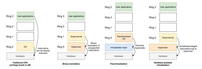
Figure 2.2: From left to right: x86 privilege levels without virtualization, binary translation, paravirtualization and hardware-assisted virtualization. Based on [59].
