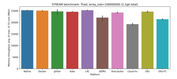
Figure A.3: Memory triad throughput STREAM benchmark
