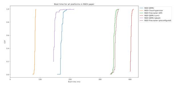
Figure 5.19: Time taken to boot hypervisors (CDF), replication of work in [3]
