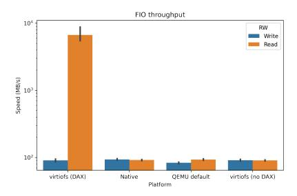
Figure 5.11: Fio virtiofs with DAX throughput (logarithmic scale)
