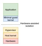
Figure 6.9: Unikernel isolation mechanism
