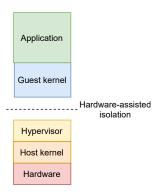
Figure 6.7: Hypervisor isolation mechanism
