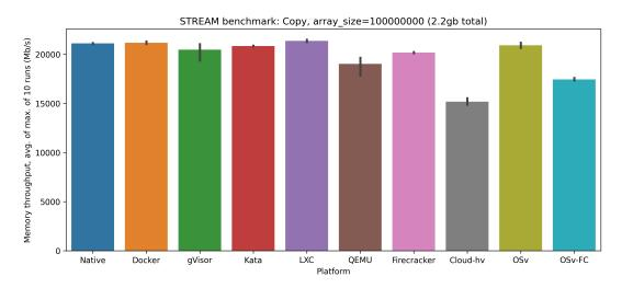
Figure 5.5: Memory copy throughput STREAM benchmark
