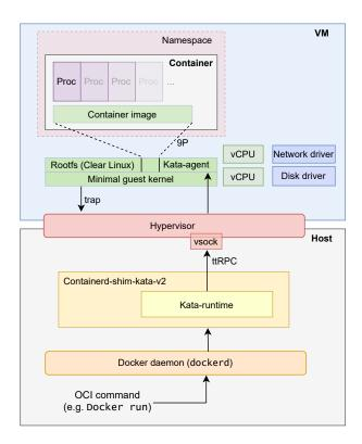
Figure 4.3: Architecture of the Kata containers secure container platform
