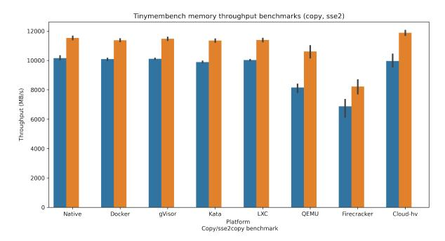
Figure 5.4: Memory throughput tinymem benchmark
