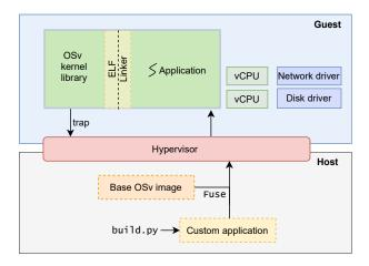
Figure 4.5: Architecture of the OSv unikernel
