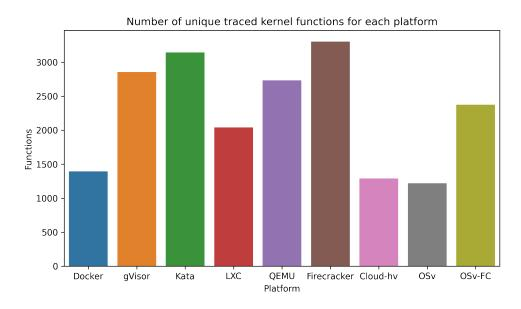
Figure 6.1: Number of unique host kernel functions executed per platform
