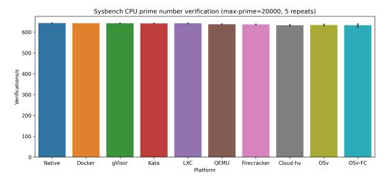
Figure 5.2: Sysbench CPU prime verification benchmark
