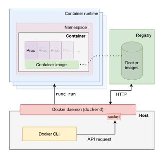
Figure 4.1: Architecture of the Docker container platform
