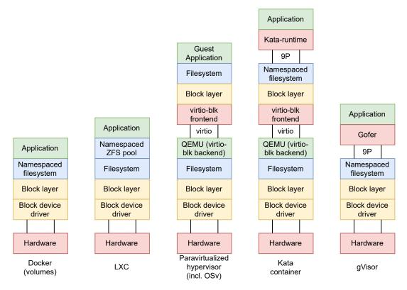
Figure 5.6: Path for I/O requests per isolation platform.
