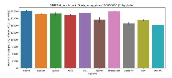
Figure A.2: Memory scale throughput STREAM benchmark
