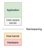
Figure 6.10: gVisor isolation mechanism
