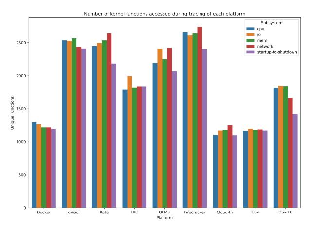
Figure B.1: Number of unique traced kernel function for each platform per workload.
