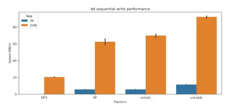
Figure 5.13: dd write throughput
