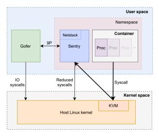
Figure 4.4: Architecture of the gVisor secure container platform
