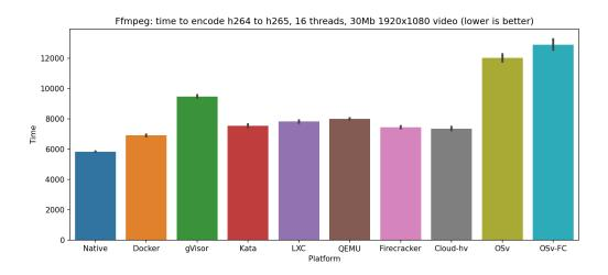
$Figure \ 5.1: ffmpeg\ video\ re-encoding\ CPU\ bound\ benchmark, re-encoding\ a\ 1080p\ 30Mb\ video\ from\ H.264\ to\ H.265.$
