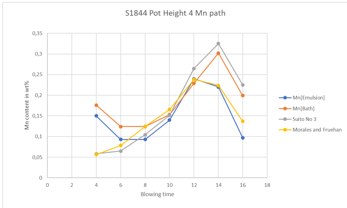
Figure C.2: Manganese partition ratio values compared with measured IMPHOS manganese partition ratio values along the time of heat S1844 in minutes. With a temperature adjustment of +50K.
