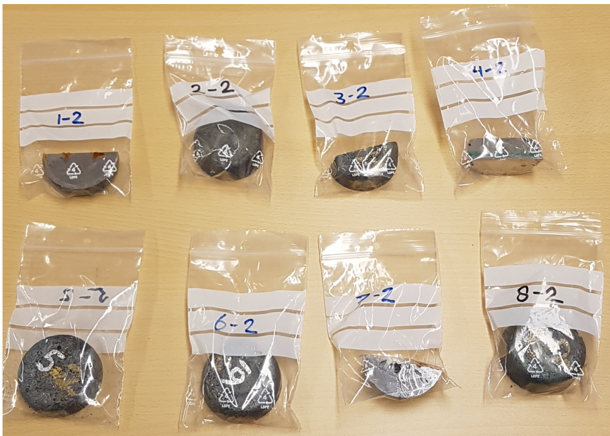
Figure 6.8: Horizontal IMPHOS samples cut 1 cm from sample bottom used for bulk chemical analysis
