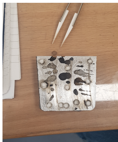
(b) Final spark OES measurement performed on whole sample
