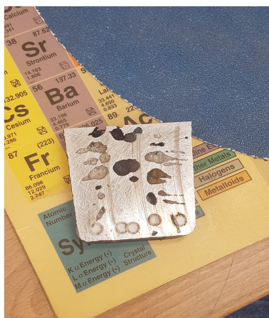
(a) Spark OES performed on bottom
