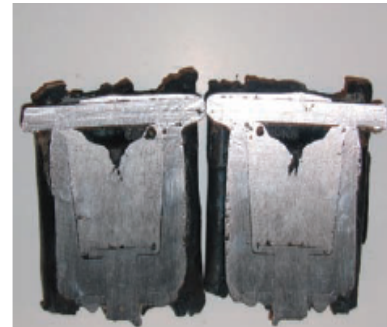
(b) Vertical cross-section of metal sample in the sampling pot (Millman et al. 2011).
