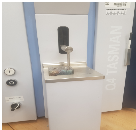
(b) Spark OES testing with sample
