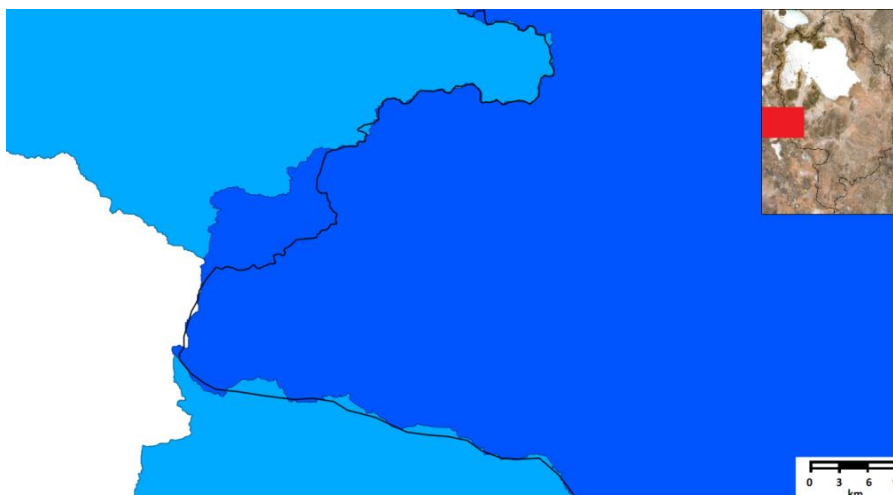
Figure 17: A part of the watersheds calculated by r.watershed in QGIS. The light blue area is the resulting watershed without inputting the location of real depressions map. The darker blue area is the resulting watershed, giving the location of real depressions map as input. The black line indicates the 'true' watershed as defined using Google Earth Pro.
