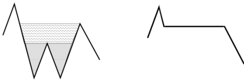
Figure 4: Filling sinks until overflow to form a filled terrain.
