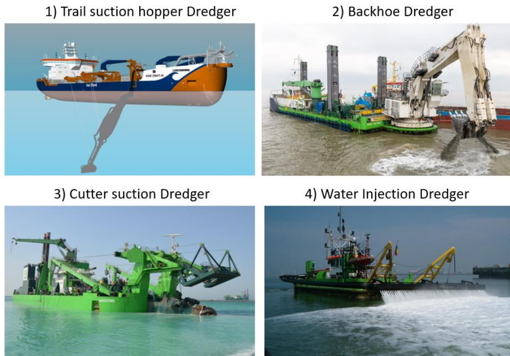
Figure 3.7: Type of dredging vessels commonly used from (DEME, 2021), (Van Oord, 2019)
