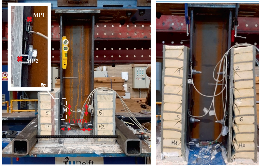
a) Final improved set-up with 4 shear connectors b) Traditional (initial) push-out set-up with 8 shear connectors
