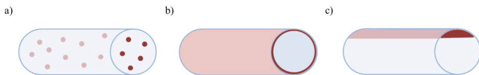
Figure 7.9. Schematic representation of a side/front view of a pipe section containing an aqueous solution of a chemical compound that a) is well mixed in the water phase, b) wets the pipe surface, and c) phase separates from the water phase.
