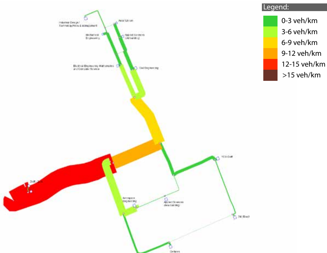
Figure 45: Density plot for the base scenario in 2 directions (35 vehicles, 18km/h)
