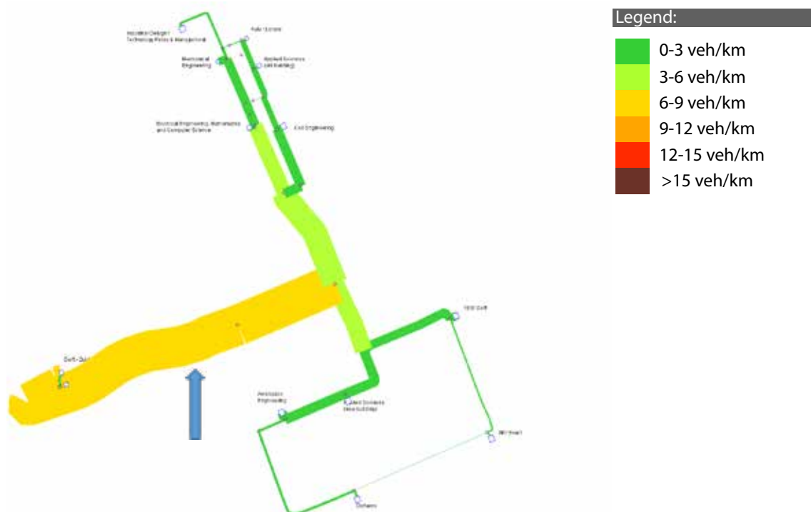
Figure 59: Maximum density plot for the scenario with removed links, 18km/h on whole network
