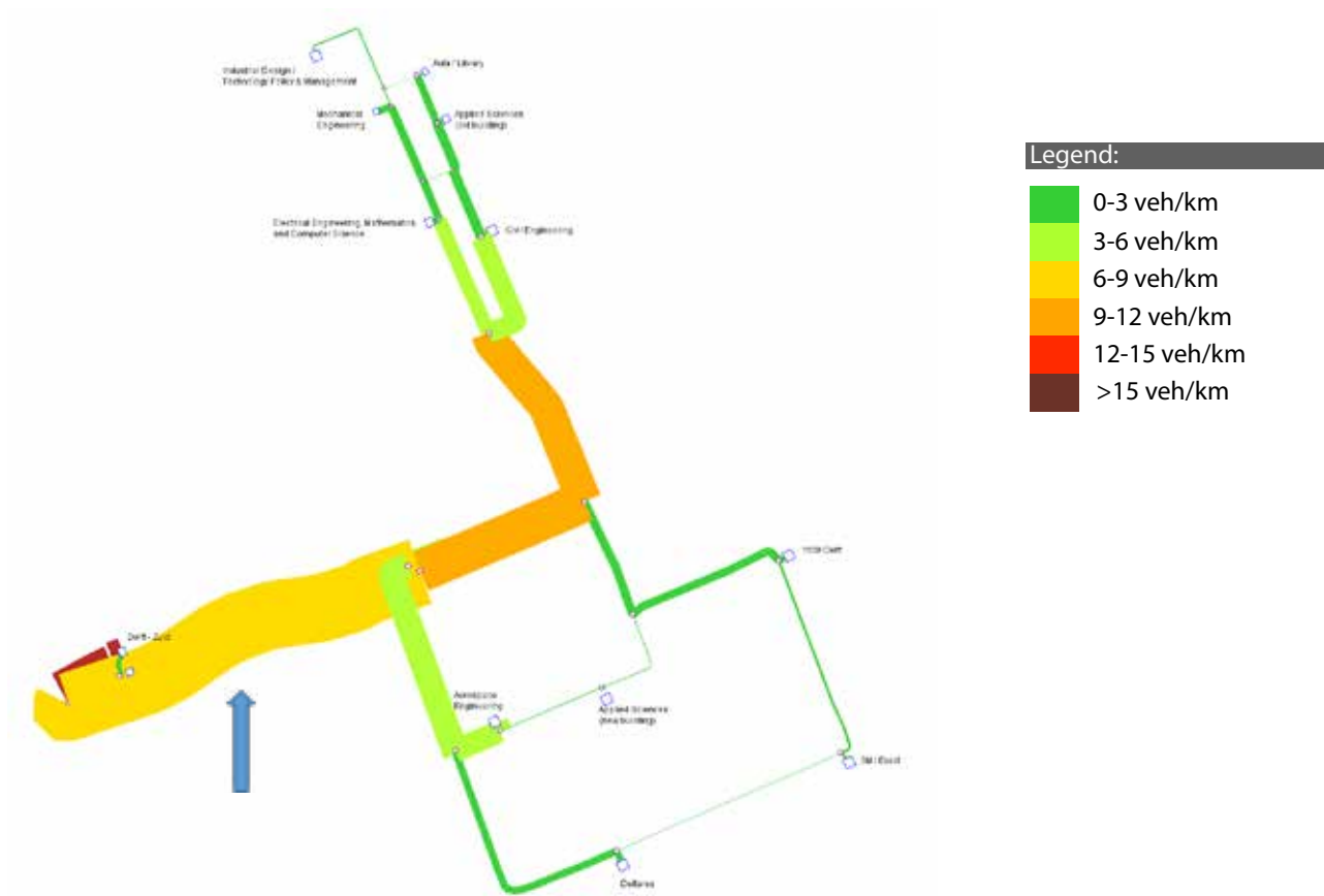
Figure 50: Density plot at 32.5 km/h on separate high speed lane (indicated with arrow)
