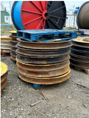
Figure 1.9: A damaged sheave, retrieved from site visit
