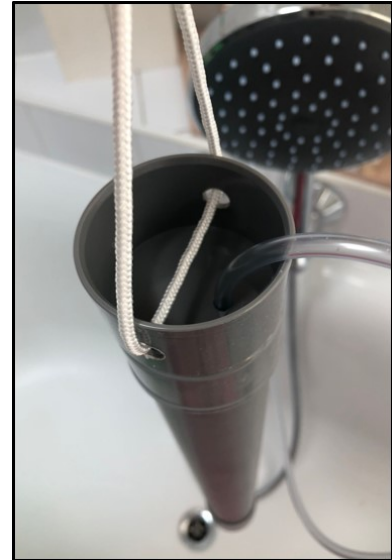
Figure 4.7: Flexible tube to facilitate water inlet at the bottom
