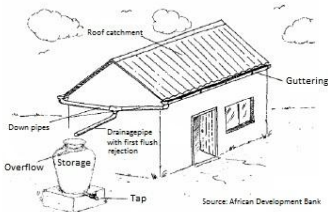
Figure 5.3 Domestic Rainwater Harvesting System
