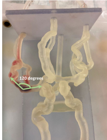
Figure 2: Patient-specific 3D printed neurovascular phantom illustrating complex arterial geometry for thrombectomy simulation [7].
