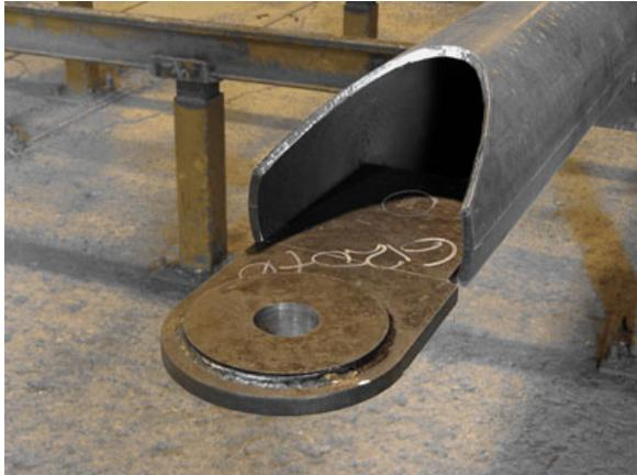
**Figure A-5: Fabrication of a pinned member**
