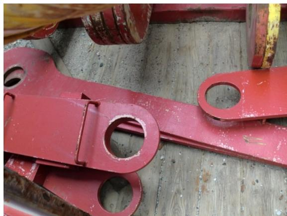
Figure A-15: Typical members for pinned connections
