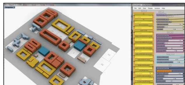
Figure 9. Example of the Graphical Interface of the tool. [Left] 3D visualization in the Rhinoceros viewport. [Right] Grasshopper window with info panels and data nodes.
