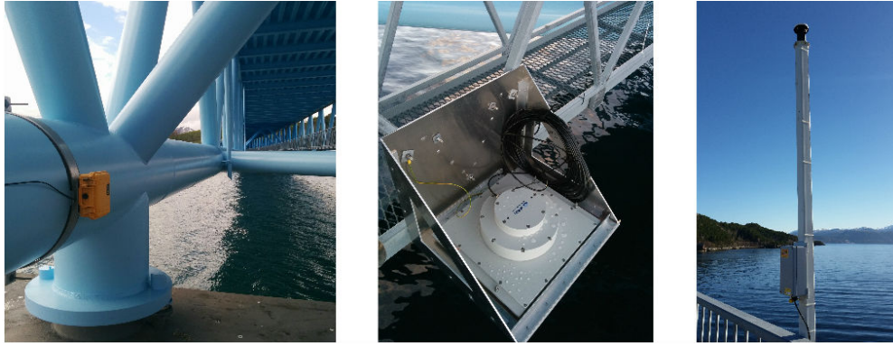
Figure 3: Selected instruments in the monitoring system. Left: accelerometer; middle: wave elevation radar; right: GNSS station. Photograph: K.A. Kvåle.
