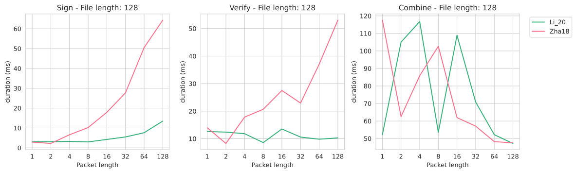
Figure 6.18: Sign, verify and combine duration of ID-B schemes - Varying packet length over a constant file length of 128.
