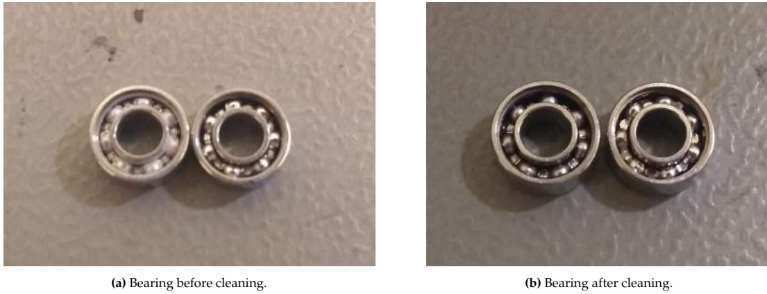
Figure 3.8: Difference in cleaning bearings.
