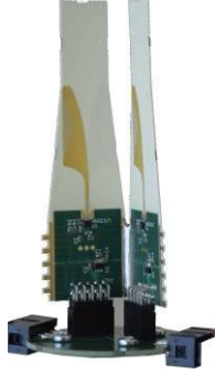
Fig. 4: Dual polarized sensing unit employed in the Antenna Dome.
