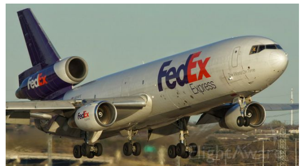
Figure 2.6: McDonnell Douglas DC-10 that uses a tri-engine set up with the third engine mounted in the vertical tail
