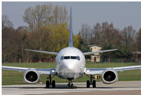
Figure 2.8: Front view of the third generation Boeing 737 classic, using the CFM56-7 engine with ovoid nacelle
