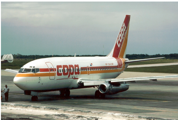
Figure 2.7: Front view of the first generation Boeing 737-200 advanced, using the older JT8D engines
