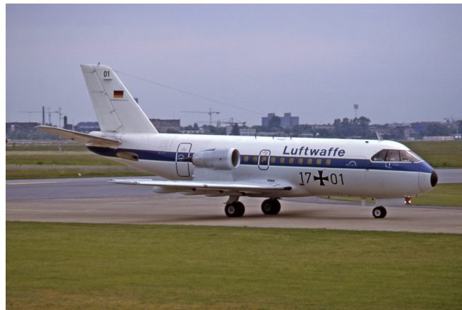
Figure 2.13: Fokker VFW 614 with over-the-wing mounted engines
