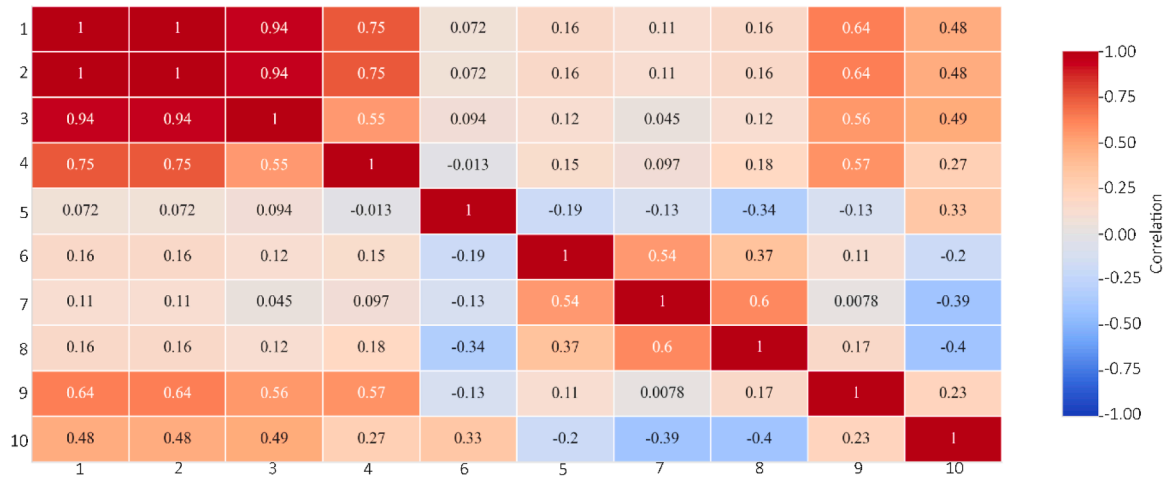
Fig. 4.1. Correlation heat map showing relationships among texture parameters, operational variables, the \delta parameter, and RR coefficient (red = positive correlation; blue = negative correlation). Axis labels 1–10 correspond to: 1 = MPD, 2 = ETD, 3 = RMS, 4 = Skewness, 5 = Tire inflation pressure, 6 = Tire temperature, 7 = Road temperature, 8 = Air temperature, 9 = Delta parameter, and 10 = RR coefficient.
