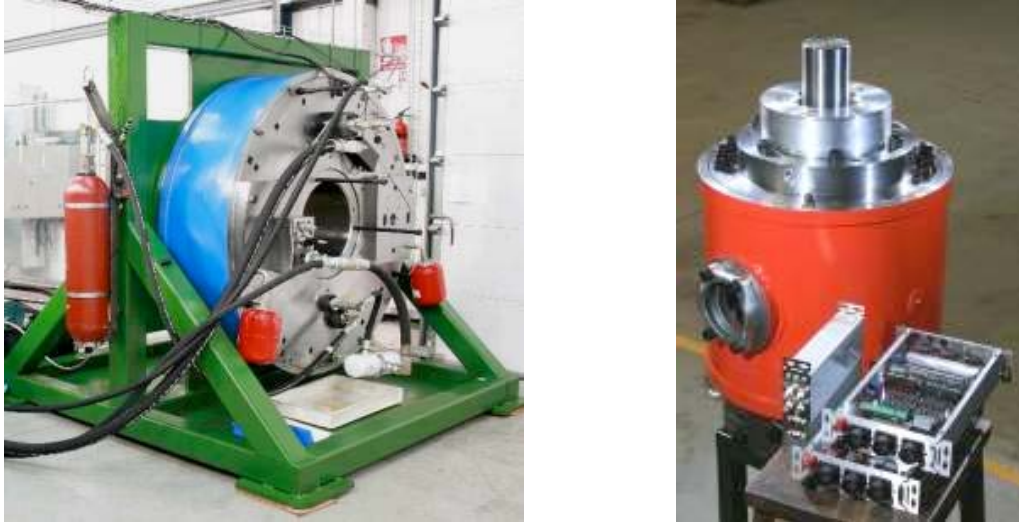
Figure 2.20 Artemis Digital Displacement 1.6 MW low speed pump (left) and 0.8 MW high speed hydraulic motor(right)
