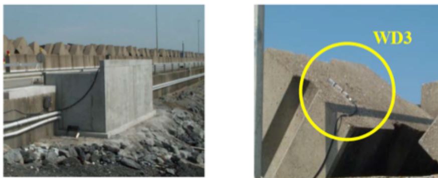
Figure 9. Detail of the overtopping tank (on the left) and wave detector, WD (on the right)
