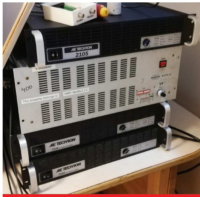
Figure 5. The current electronics setup. Black cases: gradient amplifiers. Silver case: RF amplifier.
