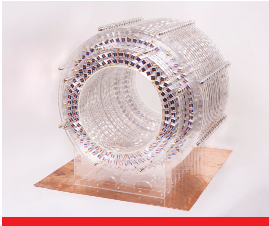
Figure 1. The current version of the low-field MRI. The picture shows the (permanent) magnet in which the patient's are inserted.
