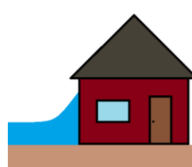
Figure 30 – Bore at the moment when the rest of the wave reaches the house
