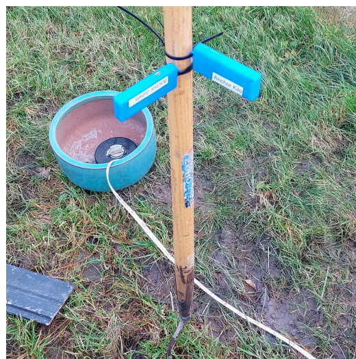
Anchor nodes on wood pole with 90 degrees offset
