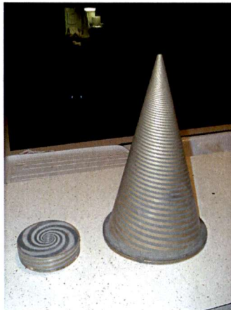
Figure 1.6: Spiral antennas for missile guidance used in the Shrike missile program
