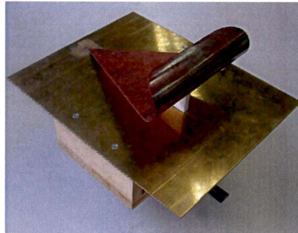
Figure 1.7: UWB horn antenna. The antenna include a rolled termination to avoid reflections and diffraction
