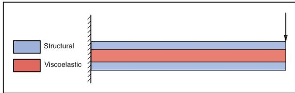
**Figure 1.** Illustration of the clamped cantilever beam containing a constrained viscoelastic layer. The arrow indicates the location of the excitation force and position measurement during dynamic loading.
