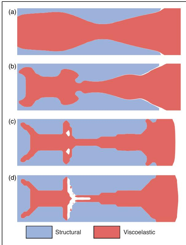
**Figure 4.** The design progression throughout the optimization routine at iteration 2, 5, 20 and 35 and the corresponding objective values. (a) Iteration 2,  $J=0.1651$ , (b) Iteration 5,  $J=0.3761$ , (c) Iteration 20,  $J=0.4553$ , and (d) Iteration 35,  $J=0.5075$ .
