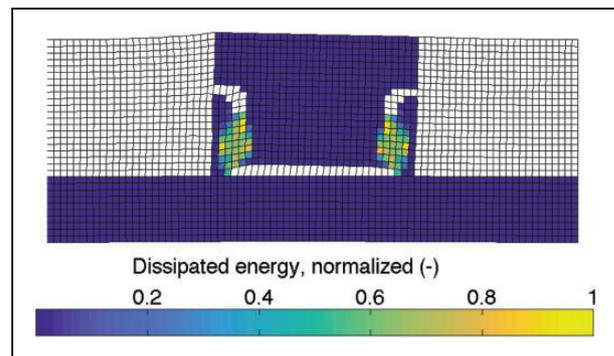
**Figure 13.** The deformation shape for the first eigenmode of the optimized structure of case study II. The dissipated energy in each element is plotted to illustrate the energy dissipation for the first eigenmode. The uncolored elements correspond to void elements in the design.
