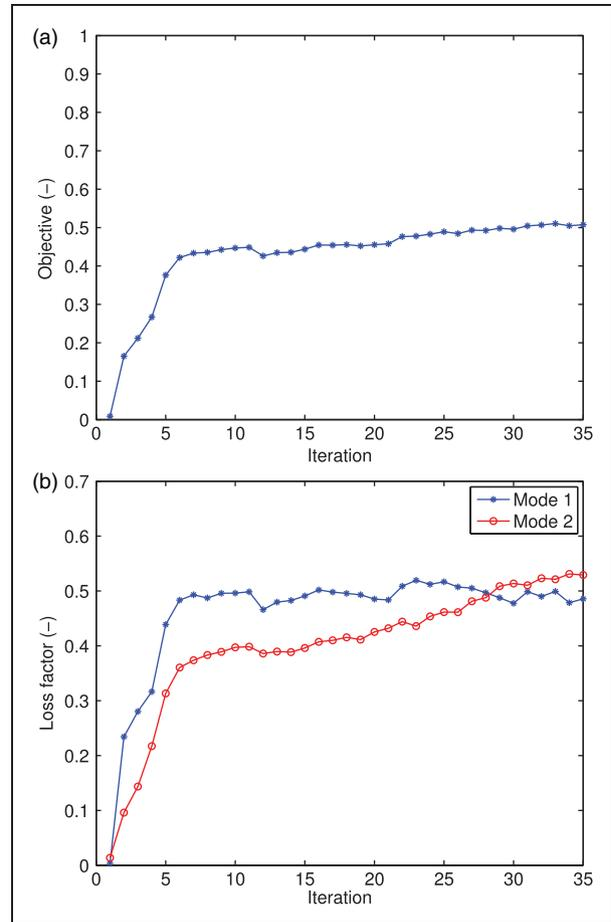
**Figure 5.** The history of the objective values (a) and corresponding loss factors (b) during the optimization.
