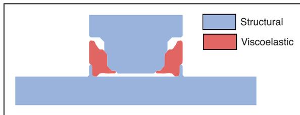
**Figure 11.** The final design of the optimization achieved after 58 iterations. The design achieved an objective value of  $J = 0.3803$ .
